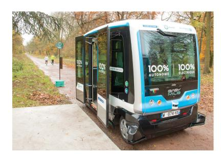
where the bus powers up in autonomous mode, exits its depot parking space and approaches the depot exit. The driver then gets on board and begins their shift. At the end of the shift, the driver leaves the bus at the depot entrance and the vehicle parks itself in the spot assigned by the automatic fleet management system. This allows for more efficient parking.
