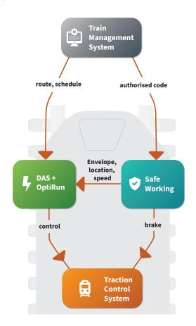
The **Traffic Management System (TMS)** is responsible for managing all the trains on a network. Each train (orange box) has a Safe working unit, a Driving Advice System (DAS) and a Traction Control System.
