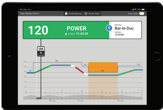
Figure 5: The display shows when the driver needs to accelerate, hold, coast and brake.
