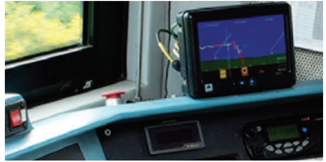
Figure 4: A touch screen in front of the driver provides real-time suggestions.
